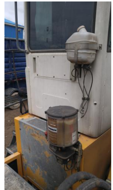
Auto-lube pumps and control systems conveniently mounted right behind the cab
